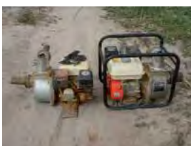
Motor pump set (1) 3,5-4,5 Hp engine, 2" pump outlet (able to pump 15-20 m3/h)
