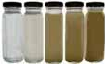
Bottles of water showing low and high turbidity
