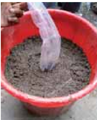
Collapse of the 'borehole' (bucket)
