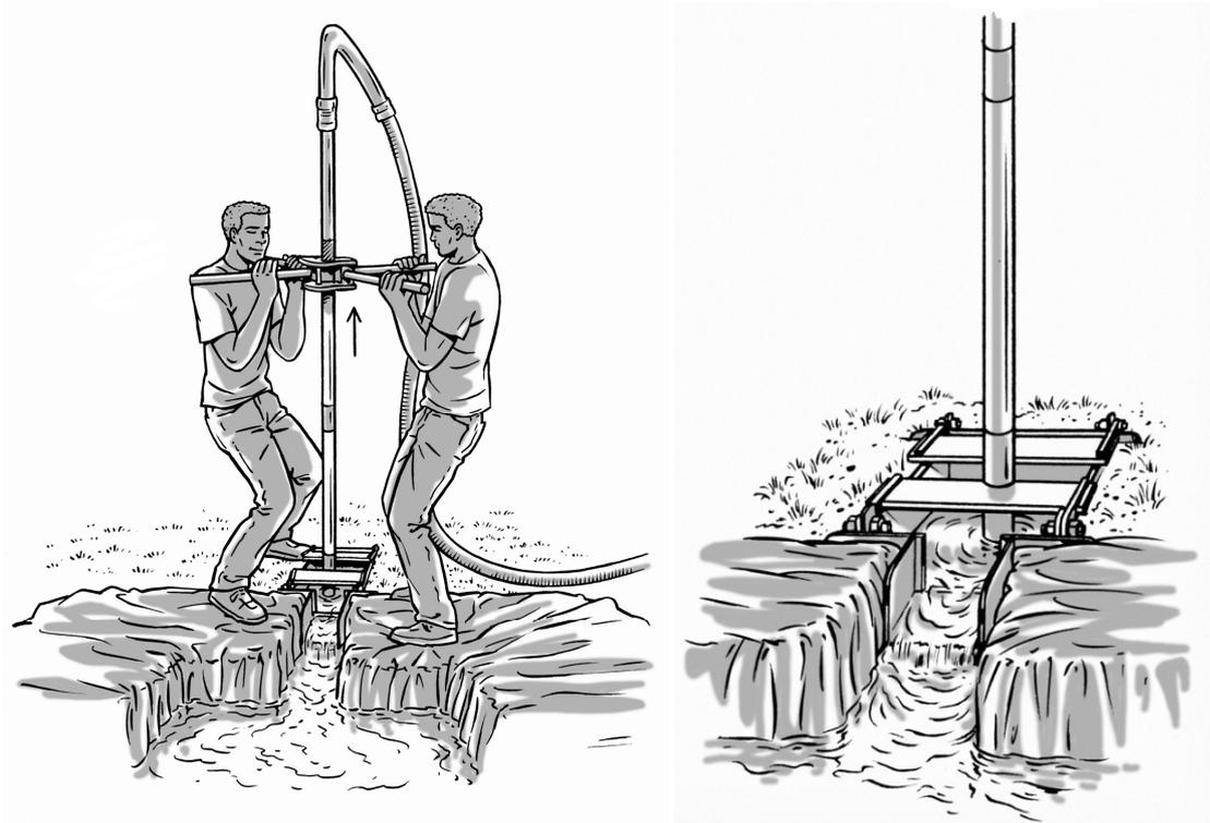
**Tip:** Keep your borehole full of water during this process! **Don't take a break now;** the chance the well collapses now is at its highest.
