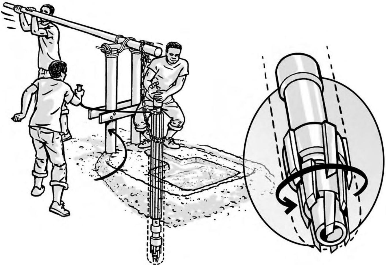
4. Move the lever down again (lift up the pipe)
