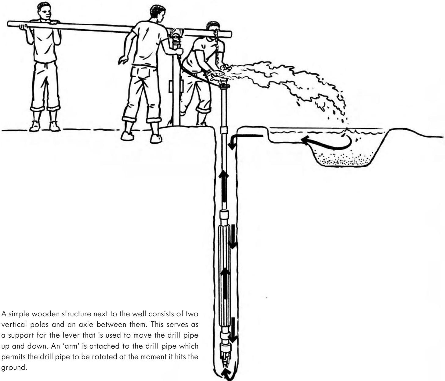
A simple wooden structure next to the well consists of two vertical poles and an axle between them. This serves as a support for the lever that is used to move the drill pipe up and down. An 'arm' is attached to the drill pipe which permits the drill pipe to be rotated at the moment it hits the ground.
