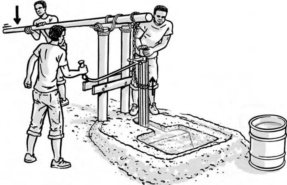
3. Push the lever up with high speed (let the drill pipe make a free fall).
