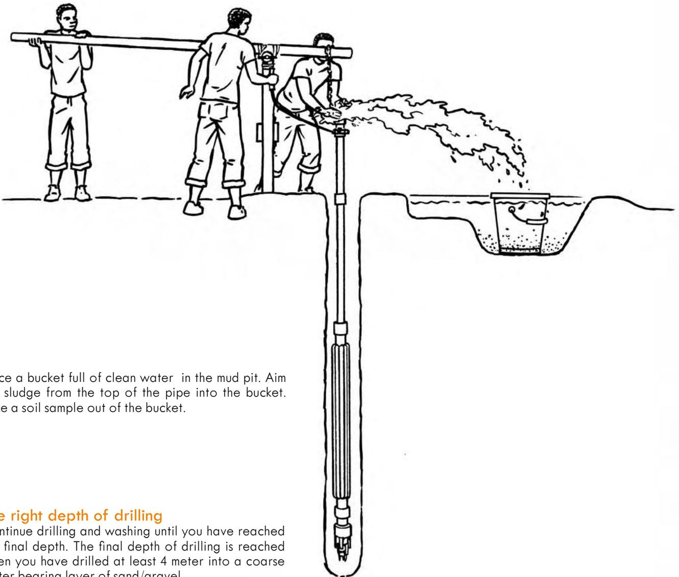
Place a bucket full of clean water in the mud pit. Aim the sludge from the top of the pipe into the bucket. Take a soil sample out of the bucket.
