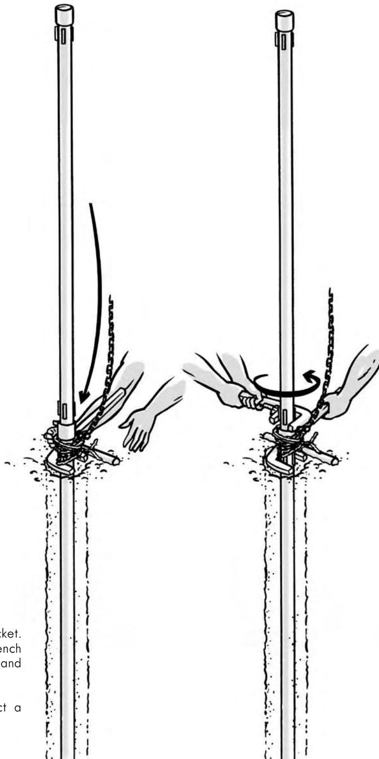
5. Place the pipe wrench under the socket. Lower the pipe until the pipe wrench holds the pipe. Remove the chain and place the chain under the socket.
