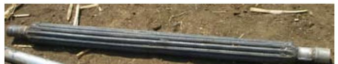
Then, weld pieces of re-bar around the normal drilling pipe, to increase the weight of the pipe. Make welds at the bottom, middle and top as shown in the picture. Two sizes of re-bar can be used;
