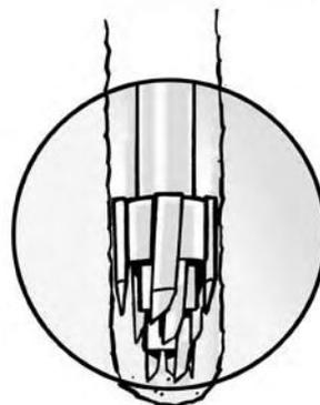
1. Move the lever up and down continuously, do not drill any deeper!
