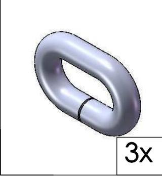
Link thickness should be between 6 and 7mm. Width should not exceed 40mm.
