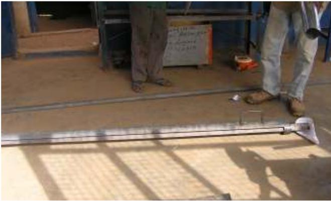
Photo 19: The pipe perforator is 2,5 m long
