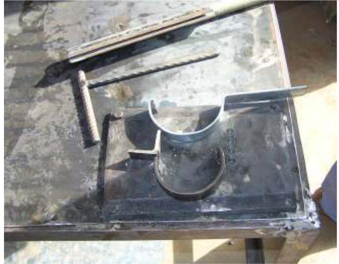
Photo 11: The product. Remark that the second bend can be made at different heights depending on the required gutter slope.
