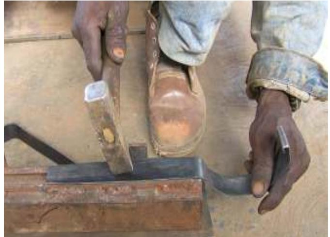
In 2007 supports are made from 2 mm not galvanized sheet and mounted **under** the roofing sheet. This is stronger and better to understand. 6
