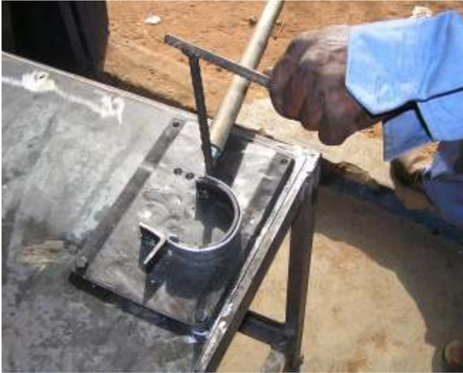
Photo 101: The pin is placed and the second bend is made.
