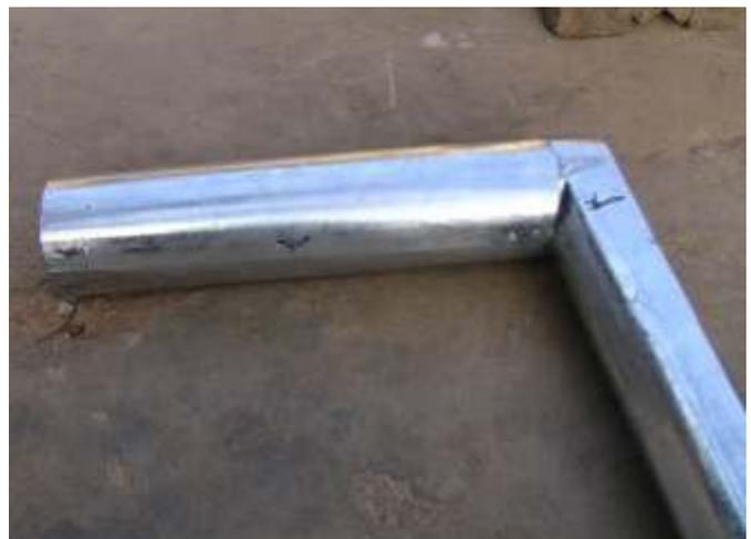
Photo 31: With the perforator two holes are punched in pipe and lip. The fourth stitch can be made.
