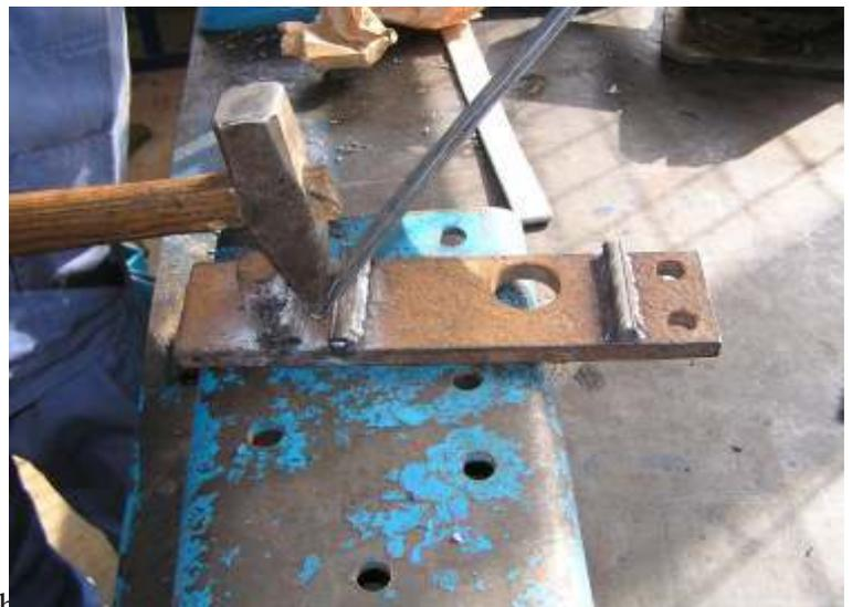
Photo 8: The end hook is bended. Remark that the photo is sun from the doubled 1 mm sheet..
