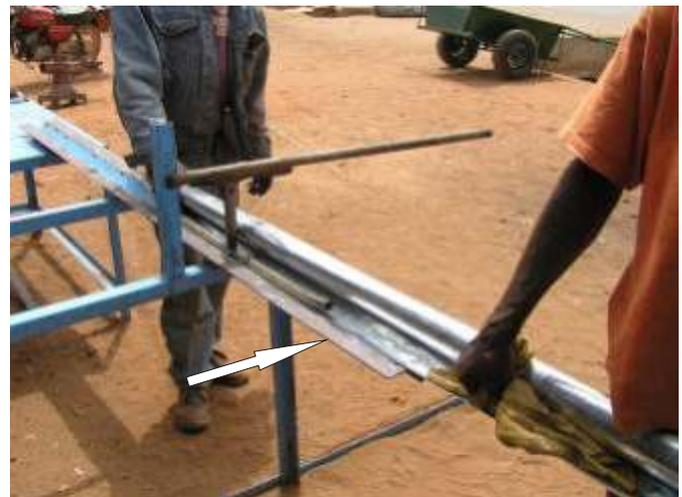
Photo 18: The pipe is rolled up at the right side.
