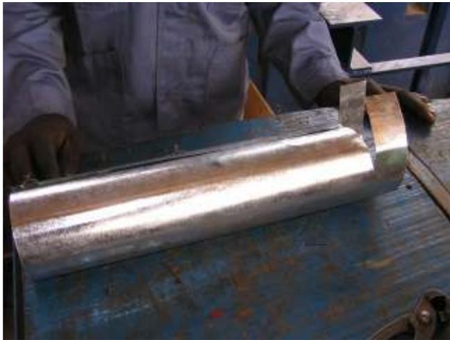
Photo 27 The pipe with two stitches
