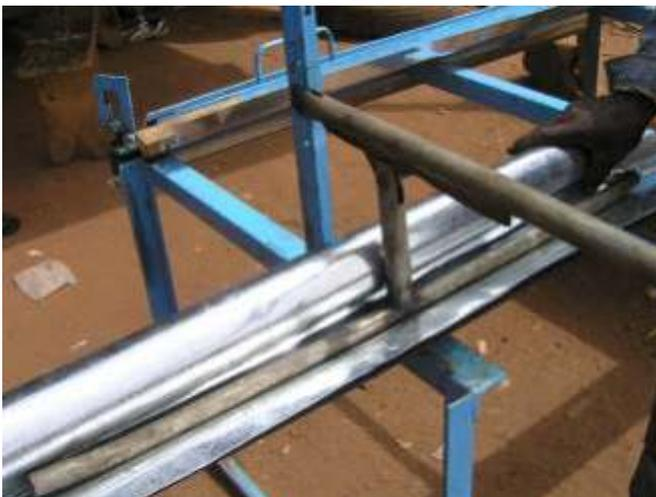
Photo 17: The pipe is rolled up at the left side.
