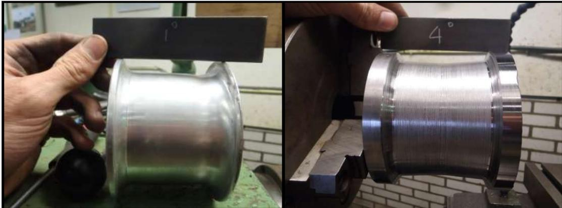
*Picture 4: Different capstan designs. Picture on left: Aluminum capstan tapered to the right; Picture on right: Steel capstan tapered to the middle.*
