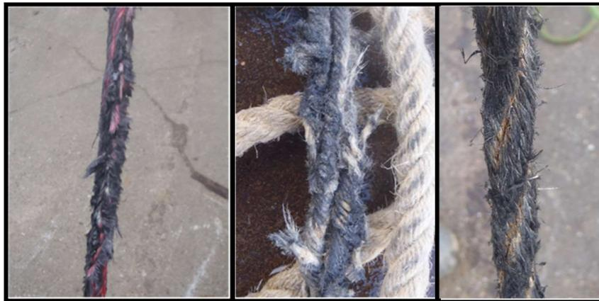
Picture 2: left to right; Damage to Samson validator, hemp, manila with same testing conditions
