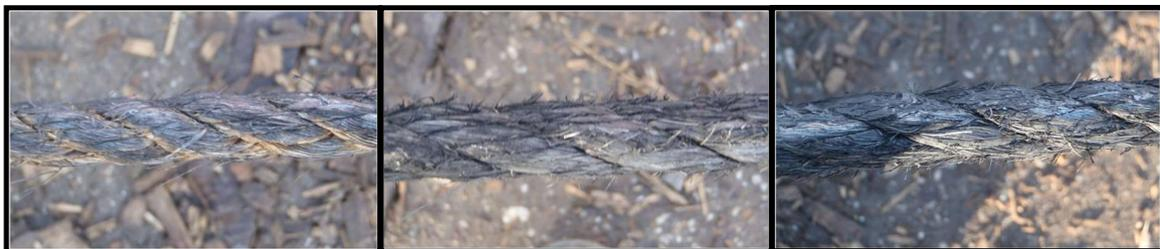
Picture 3: Manilla rope; left: 2 wraps, 76 kg, 80 rpm, middle: 2 wraps, 118 kg, 80 rpm right: 2 wraps, 160 kg, 80 rpm
