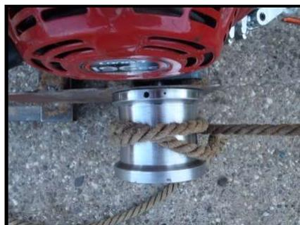
*Picture 5: Knot of rope on capstan*
