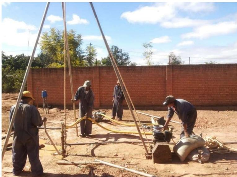
*Picture 7: Capstan combined with rotary jetting and the rotation arm of rota-sludging*
