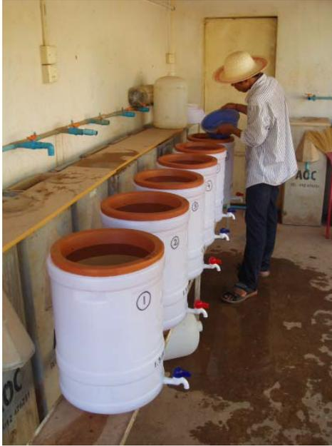
**Figure 30. Refilling of the pots throughout the constant head flow rate test**
