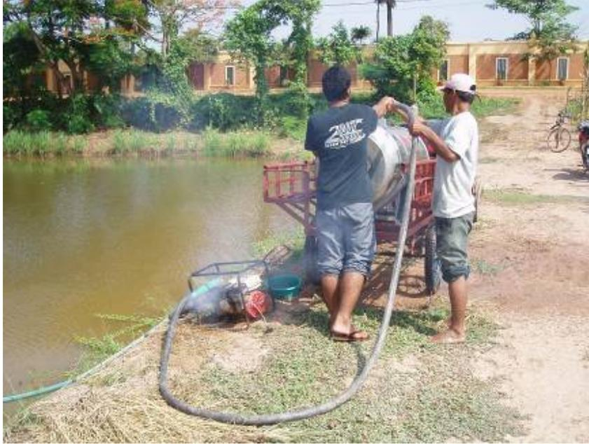
**Figure 34. Pumping of pond water for the long-term flow rate test**
