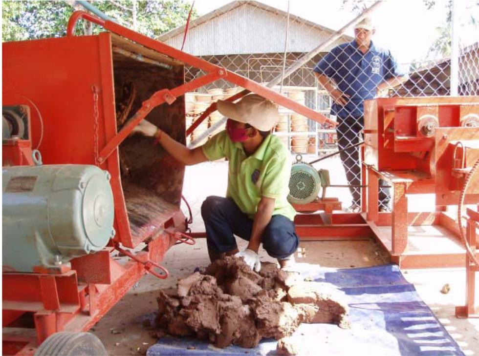
**Figure 16. Extraction of the wet mixture on the tarpaulin**
