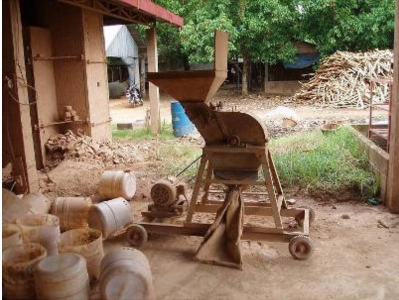
Figure 12. hammer mill used for grinding the clay and laterite
