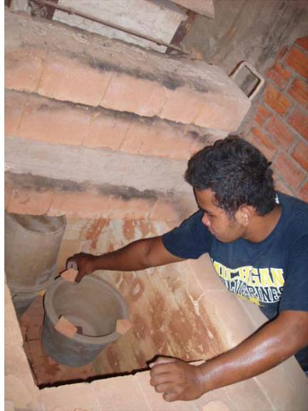
**Figure 26. Stacking of the kiln using spacers**
