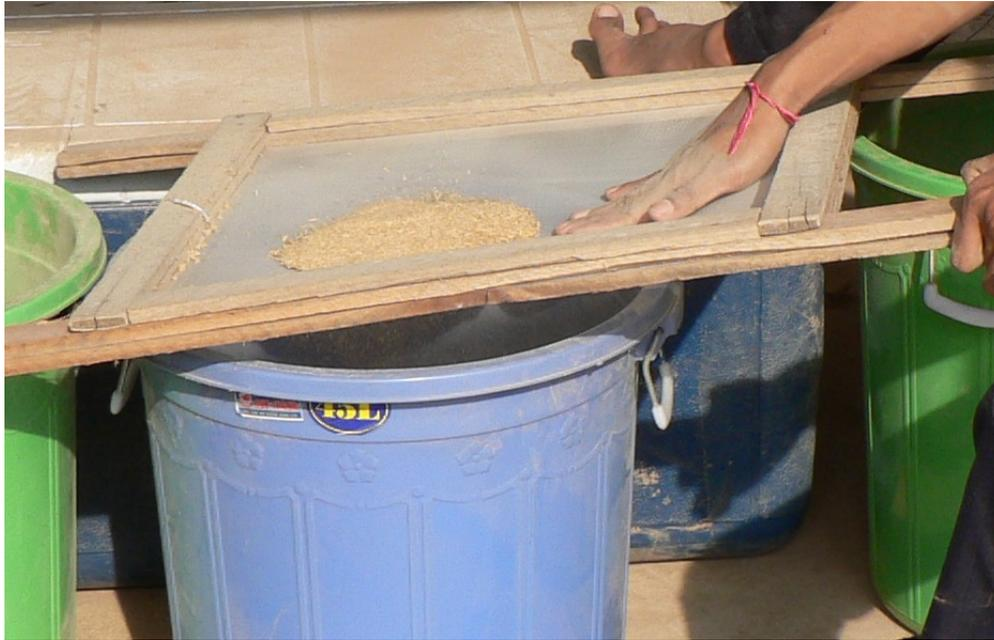
**Figure: Rice husk used for the pilot research at RDIC was sieved by hand with a sieve of 1 mm**
