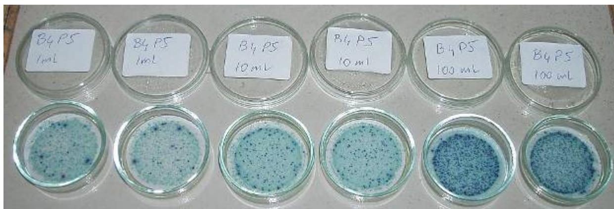
**Figure 32. *E. coli* results for 1, 10 and 100 ml duplicate effluent samples from B4 P5 without silver application (*E. coli* are purple and coliforms are blue)**
