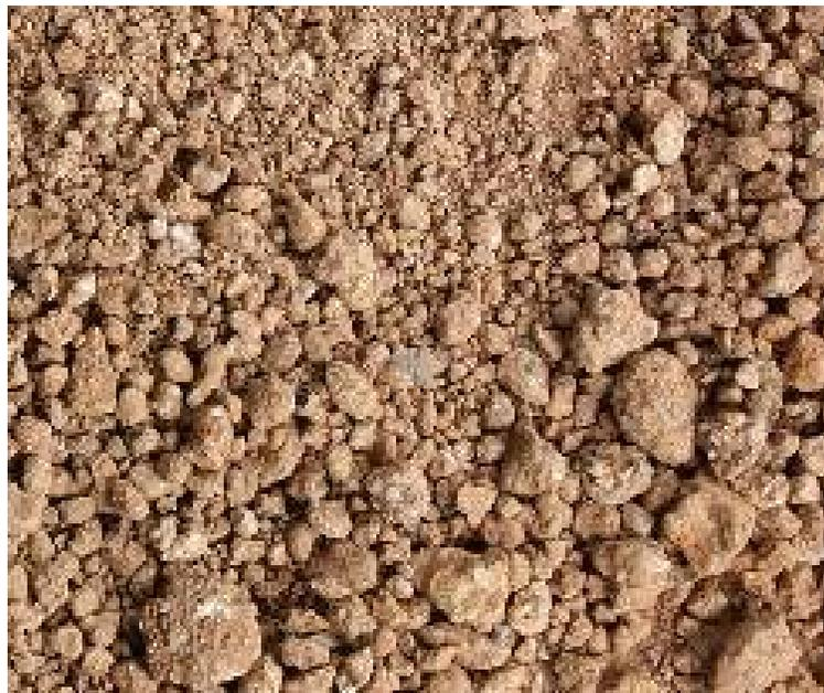
**Figure 10. Laterite sample from RDIC**
