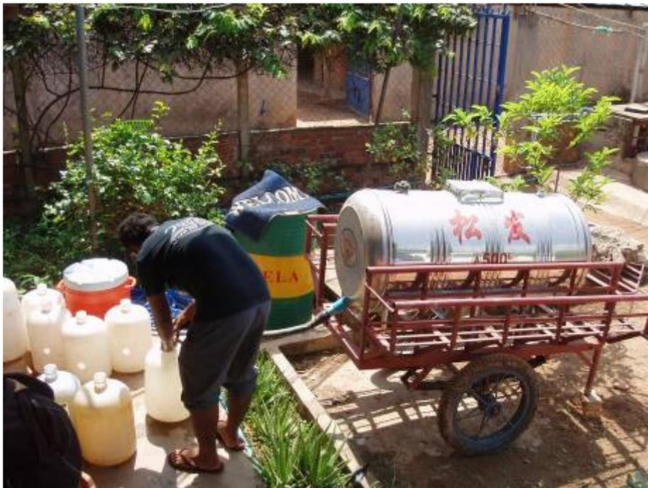
**Figure 35. Filling up 20 L bottles for the long-term flow rate test**
