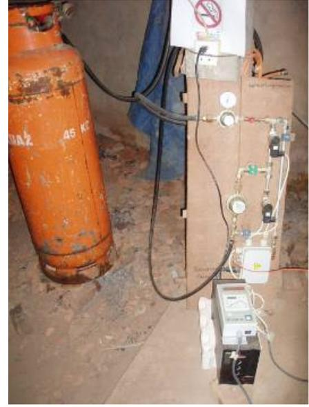
**Figure 7. Temperature regulation system for the gas-operated research kiln**
