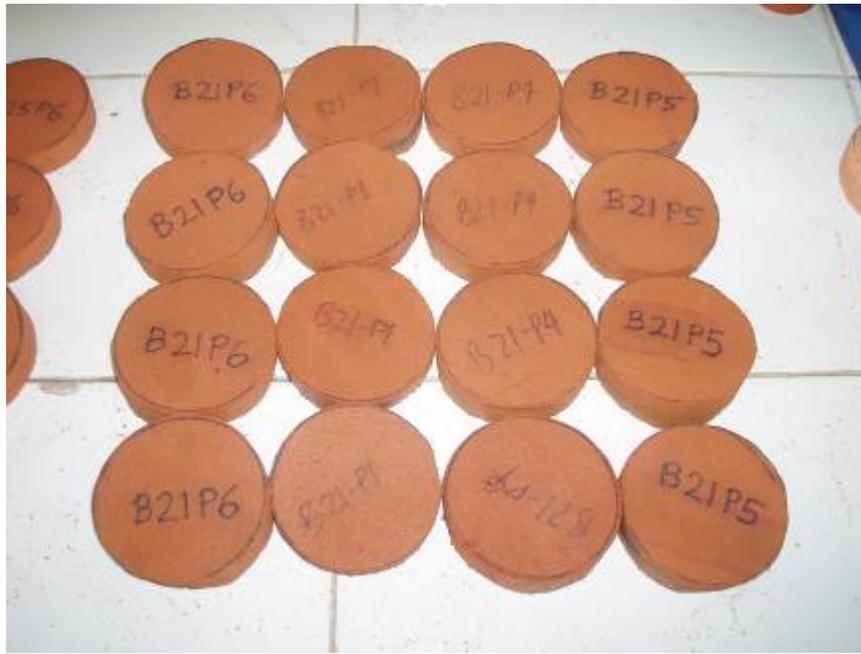
**Figure 39. Ceramic discs made from B21 P6, P1, P4 and P5**
