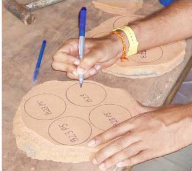
**Figure 37. Marking discs on the bottom section of a filter after the walls were broken down**
