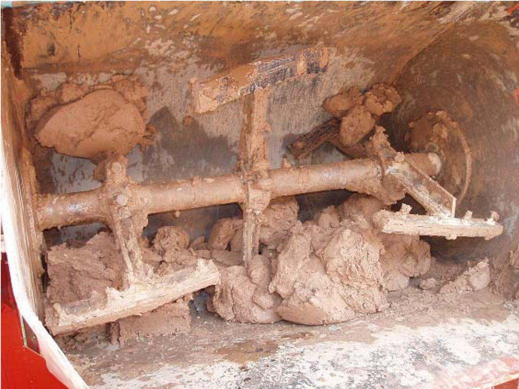
**Figure 15. Mixing of the clay mixture after water is added**
