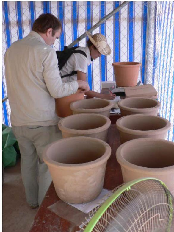
**Figure 22. Recording of the weights of batch pots during drying**
