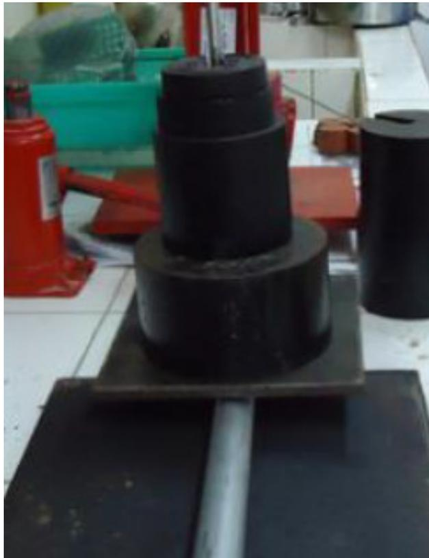
**Figure 42. Gradual loading of the lever plate with steel weights**
